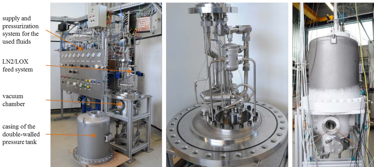
Figure 2: DLR test bench M3.3 with cryogenic injection system; left: test bench with main systems; middle: internal parts of the cryogenic temperature adjustment and injection system; right: chilled-down test bench.
