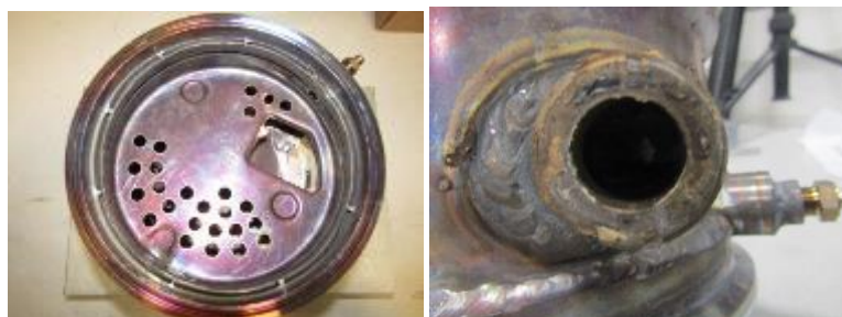
Figure 9. Images of Mixer and injector boss after the test
