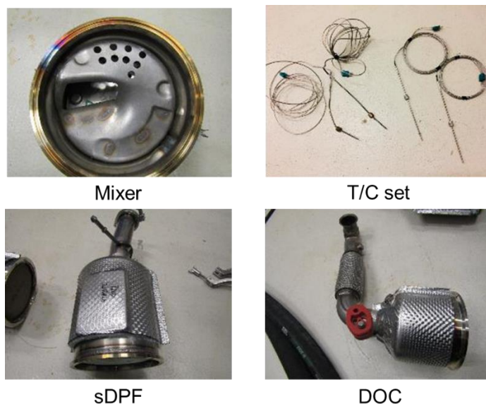
Figure 2. Deposit Test parts
