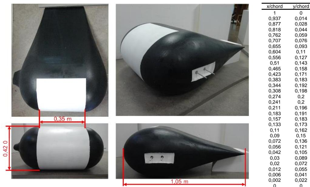
**Figure 2.** Aerofoil model views on the left. Dimensionless coordinates of the airfoil profile on the right.
