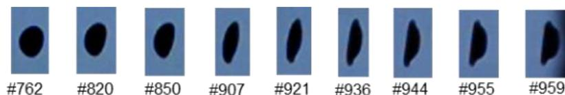
Figure 5. Droplet Evolution Images. Run 100: Droplet Diameter  $960 \mu\text{m}$ , Model Velocity 30m/s. Corresponding frames are under each image. The acquisition rate was 45000 fps.
