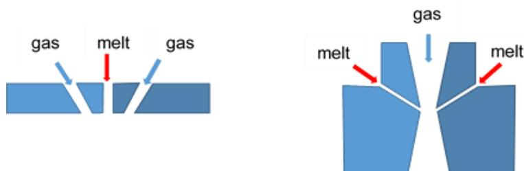
**Figure 2.** Basic difference between closed coupled atomizers on the left and the new strategy.
