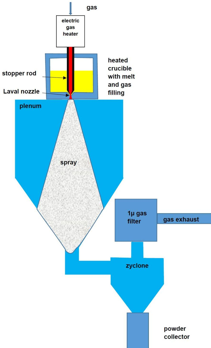
Figure 3. Schematic drawing of the experimental set-up.
