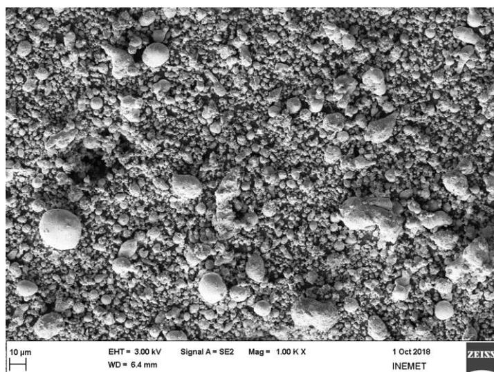
Figure 5. REM image of the tin powder.
