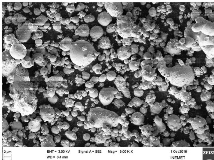
**Figure 6.** REM image of the tin powder, higher resolution.
