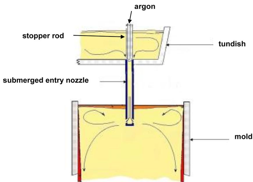
**Figure 1.** Basic arrangement for continuous casting of steel: argon is fed through the stopper rod.
