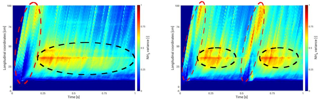
Figure 8. Comparison of  $\text{NH}_3$  CoV evolution for case 1 (left) and case 2 (right)
