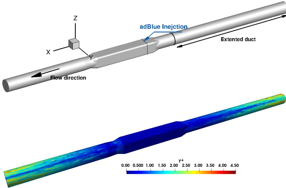
**Figure 1.** Computational domain with injection location (top) and the  $Y^+$  value along the SCR duct (bottom)
