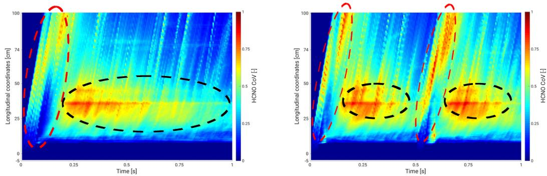
Figure 9. Comparison of HCNO CoV evolution for case 1 (left) and case 2 (right)
