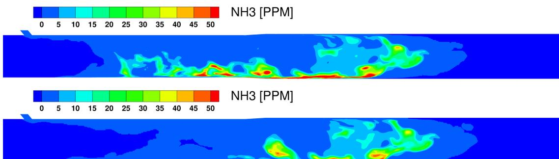
**Figure 3.** Comparison of  $\text{NH}_3$  conversion at 75 ms after SOI for case 1 (top) and case 2 (bottom)
