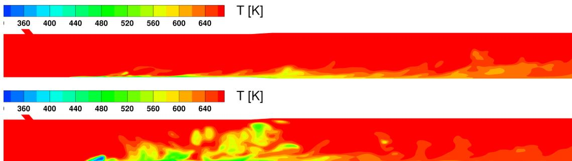
**Figure 7.** Comparison of temperature evolution at 550 ms after first SOI for case 1 (top) and case 2 (bottom)
