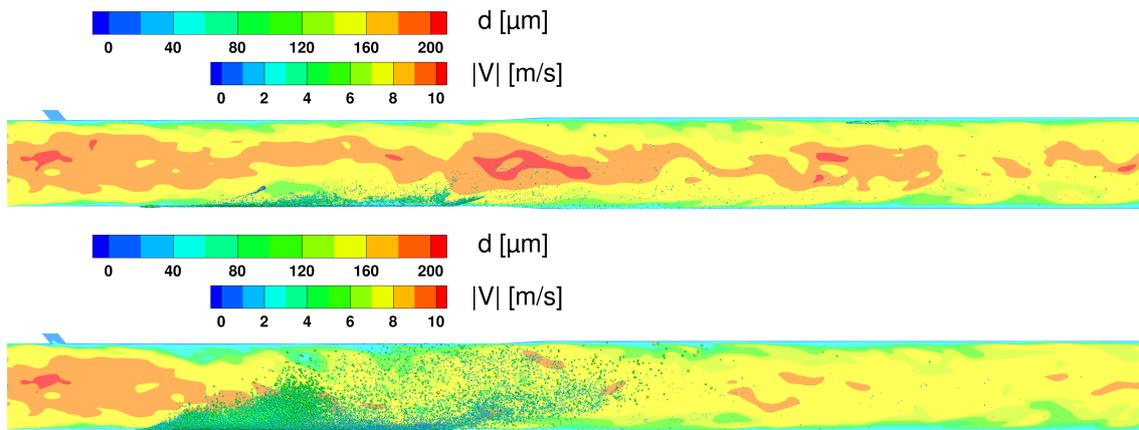
**Figure 5.** Comparison of spray and velocity profile at 550 ms after first SOI for case 1 (top) and case 2 (bottom)
