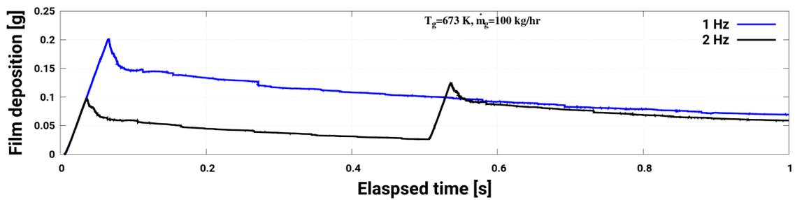
Figure 10. Comparison of adBlue deposition on SCR duct wall for case 1 (blue line) and case 2 (black line)
