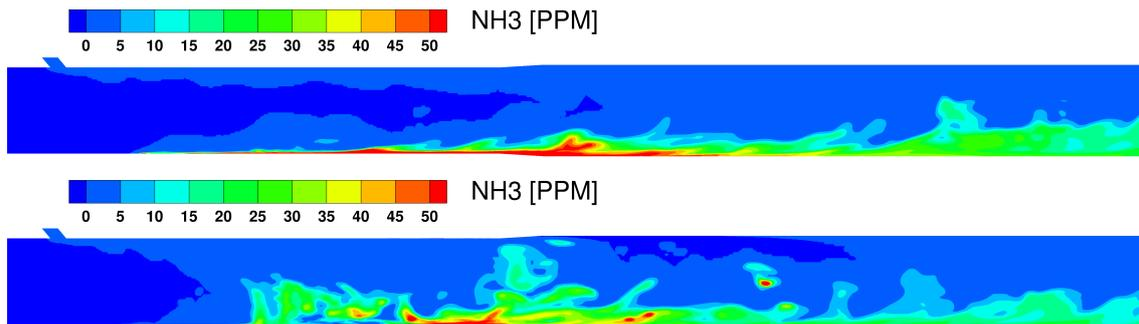
**Figure 6.** Comparison of NH<sub>3</sub> conversion at 550 ms after first SOI for case 1 (top) and case 2 (bottom)
