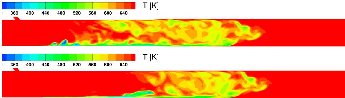
**Figure 4.** Comparison of temperature evolution at 75 ms after SOI for case 1 (top) and case 2 (bottom)
