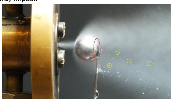
Figure 2: Spray impact on a sphere in the small-scale. Red circles: Film generation and droplet entrainment. Yellow circles: Entrained large droplets in the secondary aerosol. Sphere diameter 11 mm; distance between nozzle orifice and sphere: 5 mm; differential gas inlet pressure: \Delta p = 5 bar; feed mass flow: 2.6 kg/h. [15]
