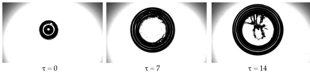
Figure 4. Sequence of images illustrating the propagation velocity of the first perturbation on the liquid film.
