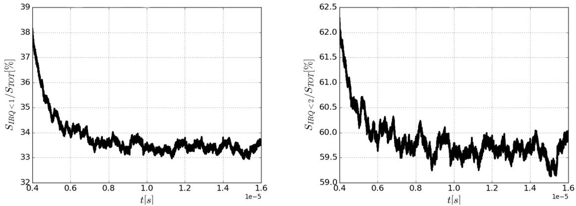
**Figure 4.** Temporal evolution of the percentage of surface with an IRQ less than 1 (left) and less than 2 (right) for the original Spray A configuration ( $We \simeq 1044$  and  $Re \simeq 70356$ ).
