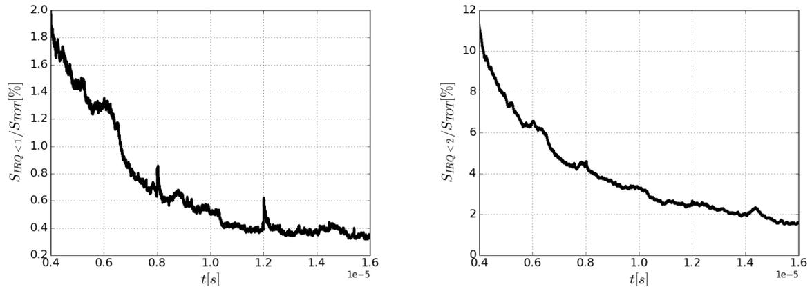
**Figure 7.** Temporal evolution of the percentage of surface with an IRQ less than 1 (left) and less than 2 (right) for the ideal Weber and Reynolds numbers Spray A configuration ( $We \simeq 2.5$  and  $Re \simeq 5795$ ).
