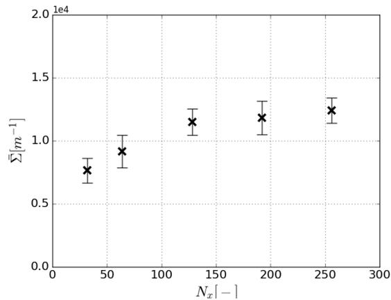
**Figure 2.** Mesh convergence of the mean surface density  $\Sigma$  for the HIT 5%. The error bars correspond to the standard deviation of the surface density value.
