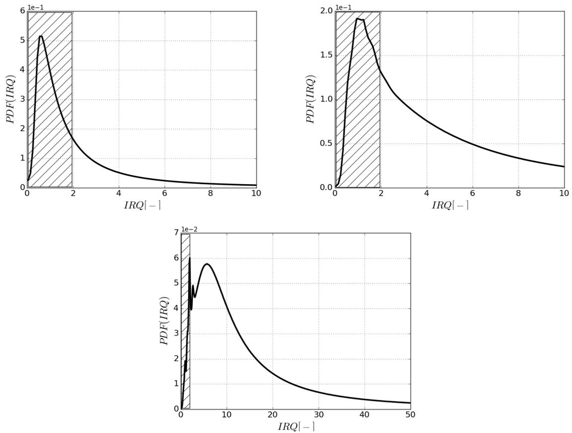
**Figure 5.** PDF of IRQ averaged in time for the original ( $We \simeq 1044$  and  $Re \simeq 70356$ ) (top left), the low Weber and Reynolds numbers ( $We \simeq 10$  and  $Re \simeq 5795$ ) (top right) and the ideal ( $We \simeq 2.5$  and  $Re \simeq 5795$ ) (bottom) Spray A configuration. The hatched part corresponds to the under-resolved zone ( $IRQ < 2$ ).
