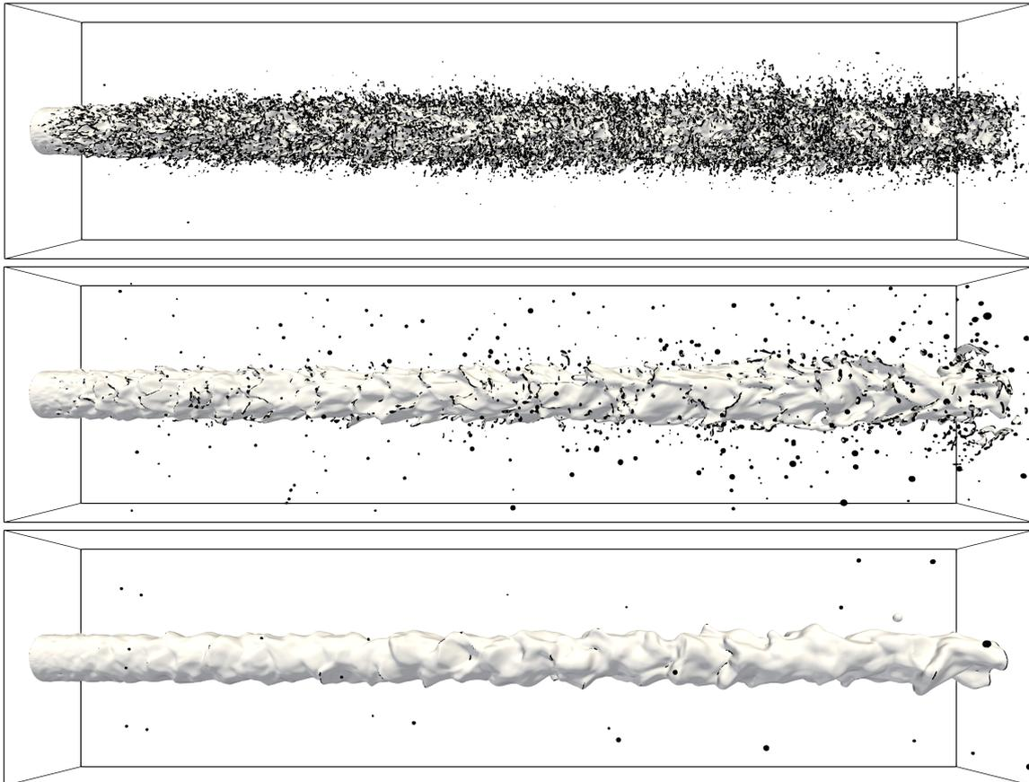
**Figure 3.** Surface representation of the Spray A configuration for high Weber and Reynolds numbers ( $We \simeq 1044$  and  $Re \simeq 70356$ ) (top), low Weber and Reynolds numbers ( $We \simeq 10$  and  $Re \simeq 5795$ ) (center) and the ideal case ( $We \simeq 2.5$  and  $Re \simeq 5795$ ) (bottom). In black, surfaces with an IRQ less than 2.
