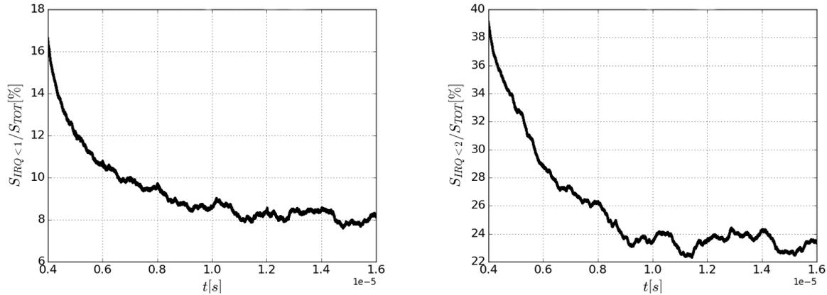
**Figure 6.** Temporal evolution of the percentage of surface with an IRQ less than 1 (left) and less than 2 (right) for the low Weber and Reynolds numbers Spray A configuration ( $We \simeq 10$  and  $Re \simeq 5795$ ).
