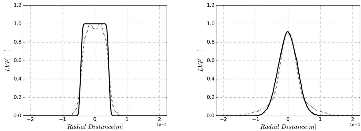
**Figure 8.** Mean liquid volume fraction radial profiles at  $1.1 D_{inj}$  (left) and  $19 D_{inj}$  (right) for the original Spray A configuration ( $We \simeq 1044$  and  $Re \simeq 70356$ ). DNS results are shown in solid line and ECN experiment, in dotted line.
