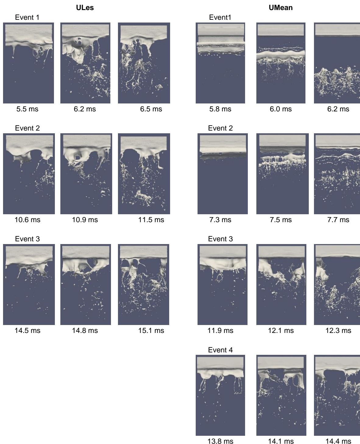
Figure 7. Liquid film evolution. Left: Influenced by turbulent velocity field from LES. Right: Time-averaged velocity profile at inlet boundaries.
