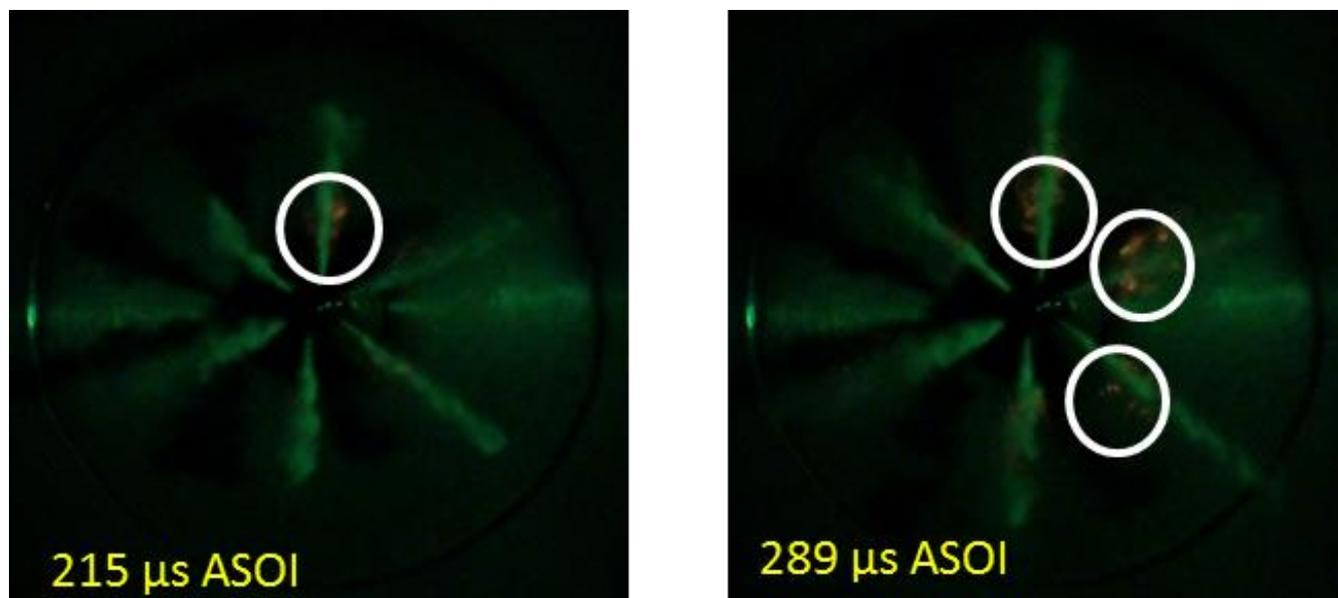
Figure 3: Location of ignition for different spray plumes from six-hole injector. Location of ignition correlates well with the location of spray bulging indicating that spray bulges create local air fuel mixture favourable for ignition.
