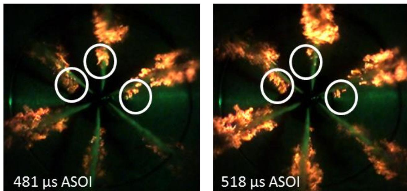
Figure 4: Images showing annihilation of flame kernels formed due to spray bulges.
