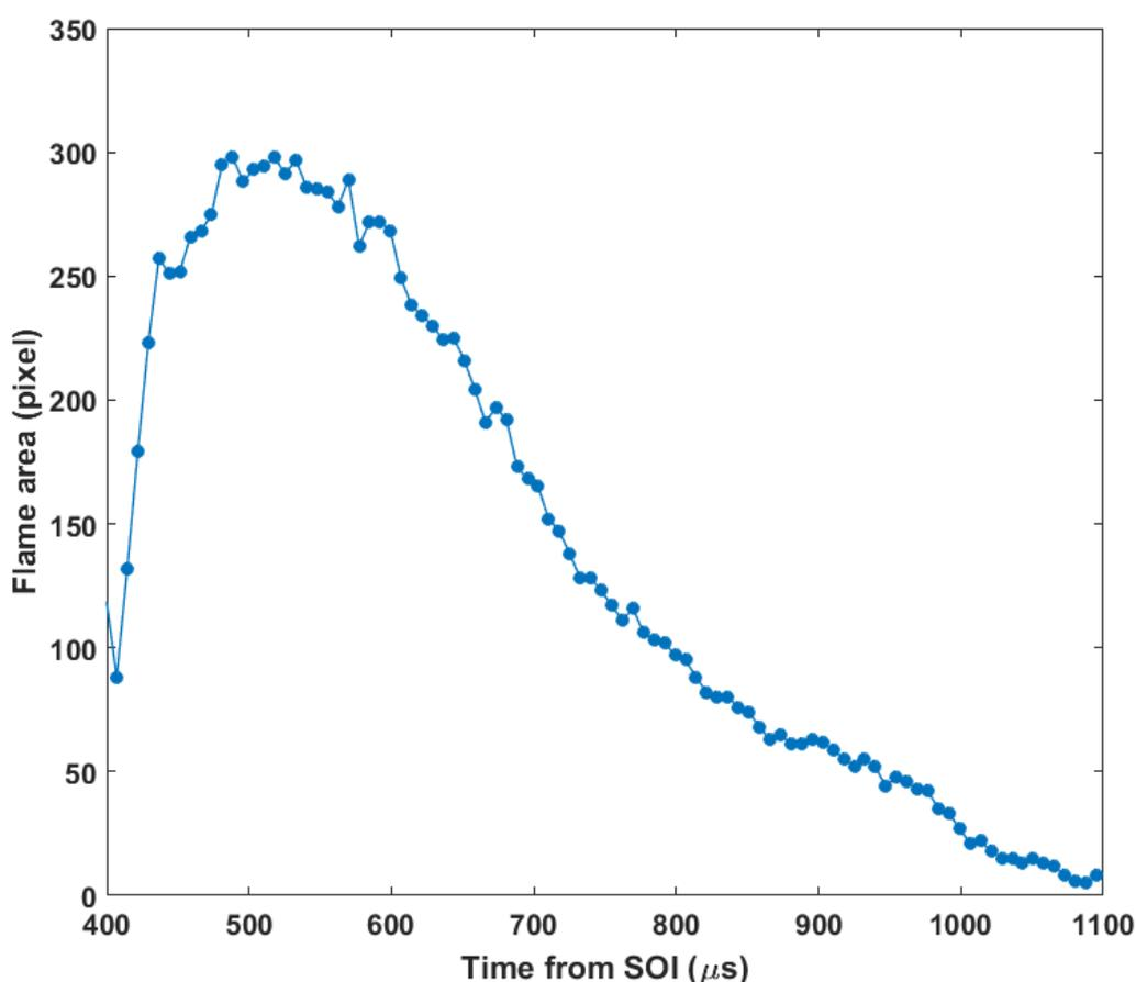
Figure 5: Variation of the flame area with time in the vicinity closer to nozzle of spray 6. Graph shows entrainment of flame pocket into the spray and complete annihilation at the end.
