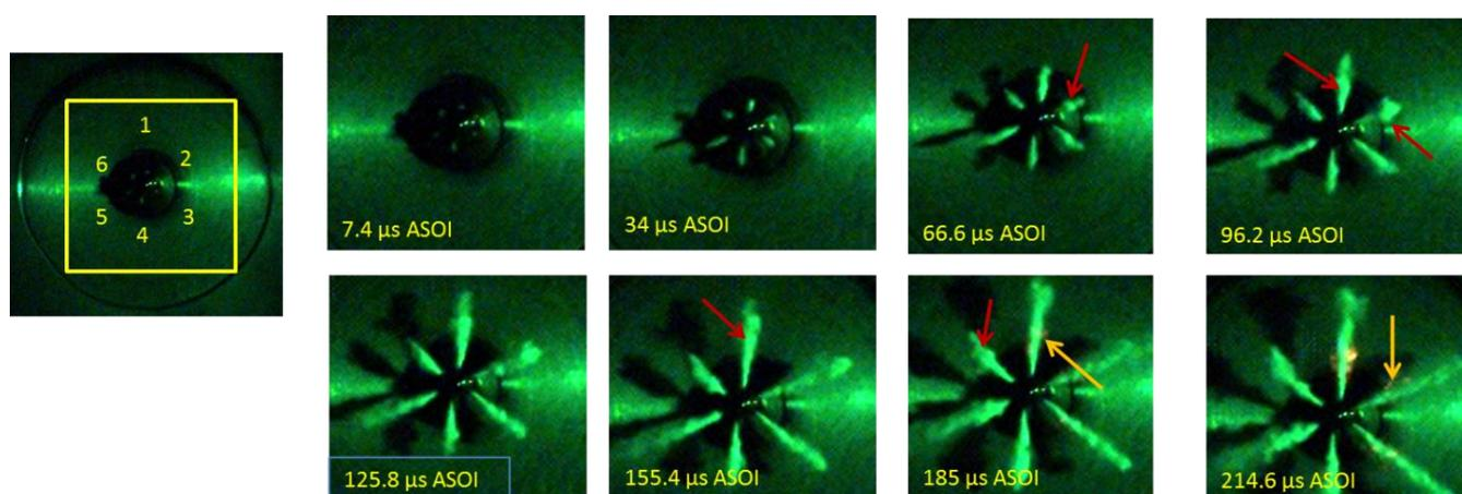
Figure 2: Local bulging in sprays during the early stages of injection.
