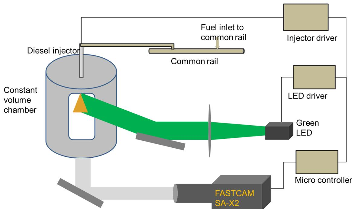
**Figure 1:** Schematic of experimental setup used in present study. Spray was illuminated using LED and spray combustion images inside constant volume chamber were captured using a high speed camera. Synchronization of injection, LED and camera was done using a controller.
